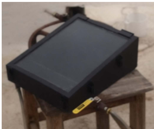
Figure 2: Solar reactor for the accelerated fermentation of Carbohydrates to hydrogen proposed to be fabricated using carbon fiber reinforced composite (CFRC)
